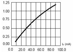
Relative Luminous Flux vs Forward Current
