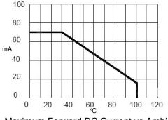
Maximum Forward DC Current vs Ambient Temperature
